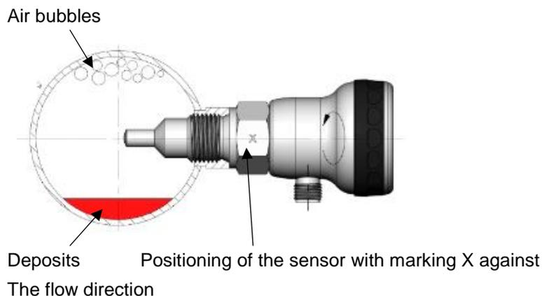
Fig. 1: Air bubbles on probe
