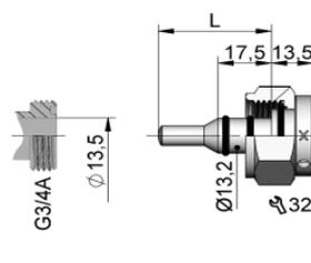
Push-in sensors with system mounting are mounted in the pipeline using a system T-piece (accessory) or a system welding or soldering socket provided for this purpose.
