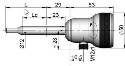
Push-in sensors with variable immersion depth are mounted in the pipeline using mounting fittings provided for this purpose.
