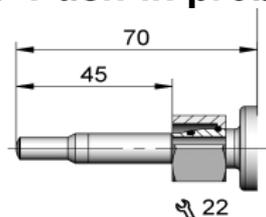
Insertion probe with defined immersion depth. The M18x 1.5 union nut is screwed onto a suitable socket on the pipe side. Torque max. 40 Nm. Sealing is achieved via the 24° sealing cone. Depending on the T-piece used, this type of mounting allows a pressure load of up to 100 bar.
