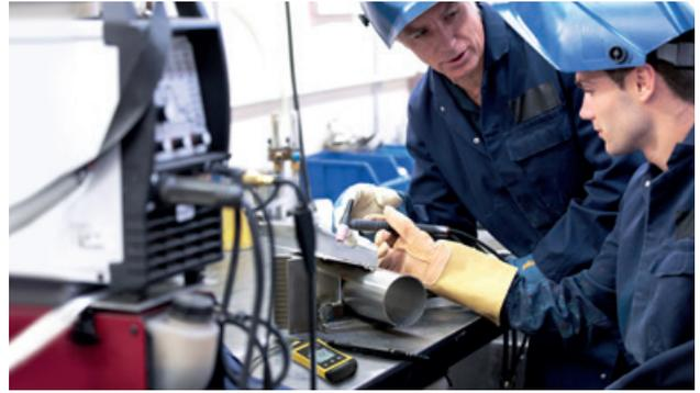
In many industrial processes temperature is one of the most important parameters. For example, measuring the surface temperature within split seconds before the welding process. Fast surface measurements on metal surfaces are the strength of the G 120x and its matching surface probes.
