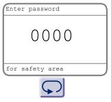
Entry of the password for the security level (0010 in condition as delivered)
