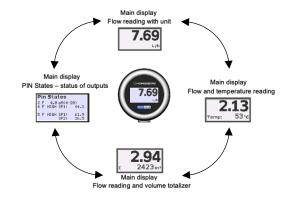
The measured flow value is shown with the unit as the start display. *RING TURN* displays a main page at a time. You can effect sub-actions with RING SHIFT for 2 seconds.
