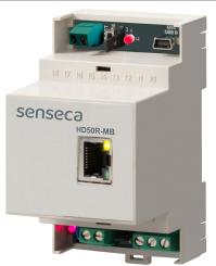
Data logger with **Master** RS485 Modbus-RTU interface for acquiring sensors with RS485 Modbus-RTU output (for example an anemometer of the HD52.3D... series). A voltage-free contact input allows connecting a rain gauge with contact output.
