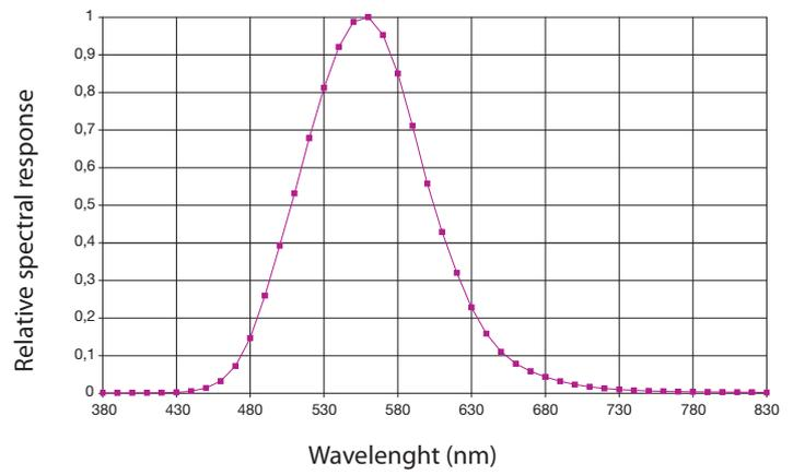
Figure 7 - HD2021T6 probe relative spectral response
