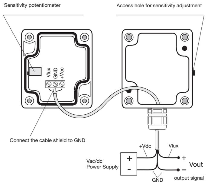
Figure 4 - Connection diagram for HD2021T... with voltage output
