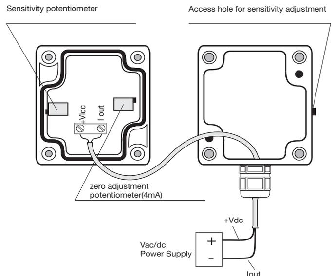
Figure 5 - Connection diagram for HD2021T... with current output
