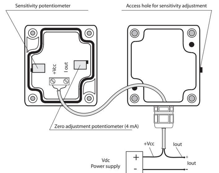
Fig. 2 - Connecting diagram with current output
