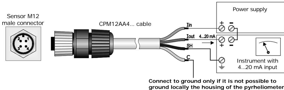
Fig. 4.2: LPPYRHE16AC connections
