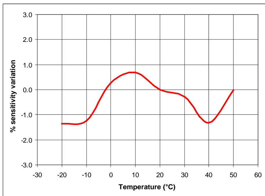
**Fig. 2.1: % variation of sensitivity of the LPPYRHE16 pyrhelimeter with regard to sensitivity at 20 °C in the temperature range from -20 to 50 °C**
